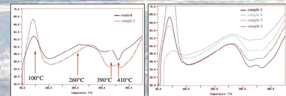
Fig. 13-14. Differential scanning calorimetric (DSC) measurements of the samples. 100°C – water; 260°C – hemicellulose deg.; 390°C – cellulose deg.; 410°C – polymerisation of the degradation products.
